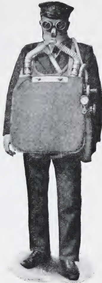
FIG. 56.—THE FLEUSS APPARATUS FOR USE IN MINES. (SIEBE, GORMAN AND CO.).
